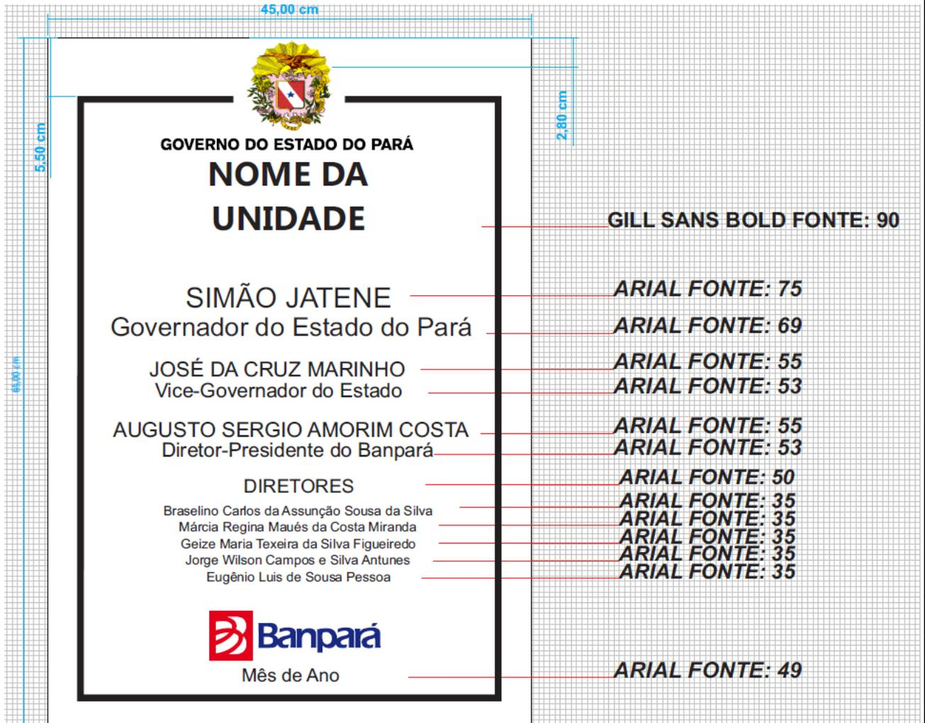
The image shows a layout for an inauguration plaque. The overall dimensions are 45.00 cm wide and 5.50 cm high. The plaque itself is 45.00 cm wide and 2.80 cm high. The text is centered and includes the state coat of arms at the top. The text is as follows:
